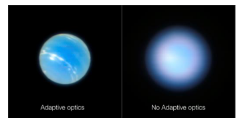
Images of the planet Neptune obtained with MUSE/GALACSI instrument on ESO's VLT (left hand side: Adaptive Optics control in loop, right hand side: no adaptive optics correction, source: ESO)
