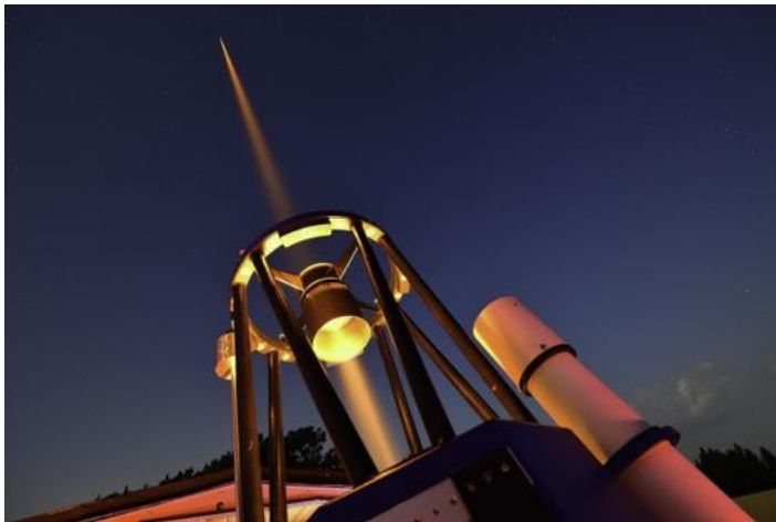
Twilight operation of the OSL Sodium Guide Star Laser system
